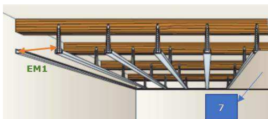
Figure 5 - Fixation de la plaque PREGY XL BA13
